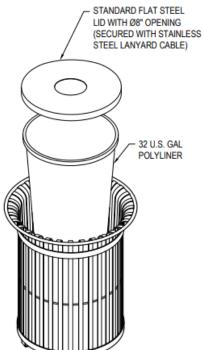
The classic flared top with steel slat design is an ideal option for parks, offices, and city streets. The steel lid is tethered to the receptacle to prevent theft and vandalism. Featuring all-steel, fully welded construction with a powder coat finish for rugged durability. The polyethylene liner permits easy waste removal and cleaning. Model 223-32D has a latching and lockable door to simplify liner removal and cleaning (padlock not included).
